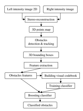
Figure 1. Obstacle classification system architecture
